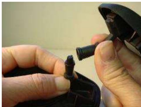
Figure 44: Connecting Speaker Pod to Wiring Loom.
