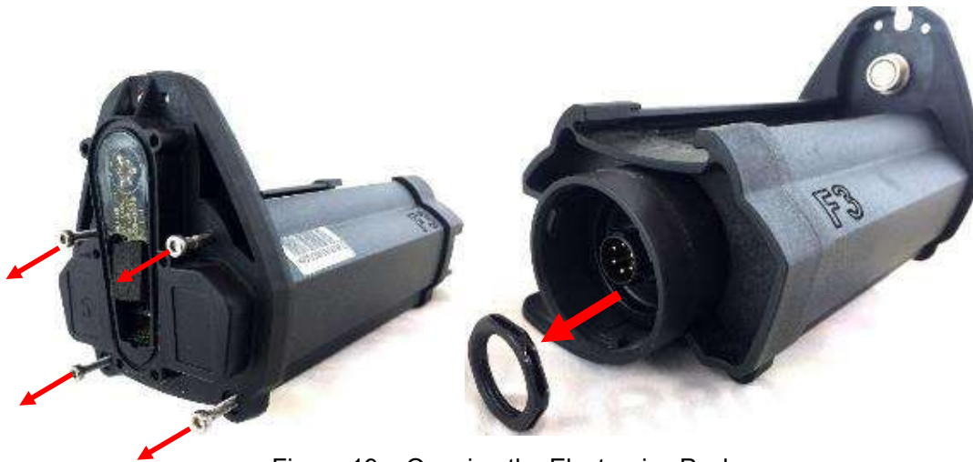
Figure 19: Opening the Electronics Pack
