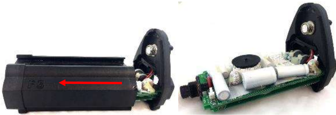
Figure 21: Removing the Electronics Pack housing.
