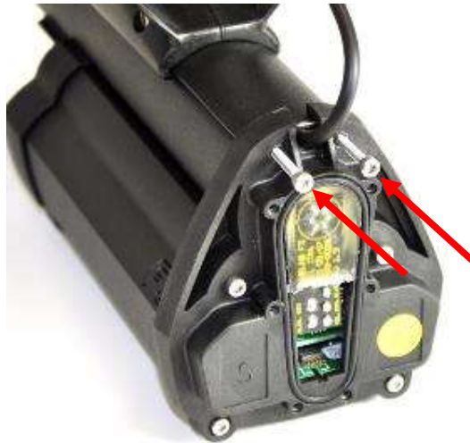
Figure 55: Connecting the Electronics Pack to the shaft.
