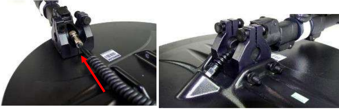
Figure 38: Attaching UXO Coil.
