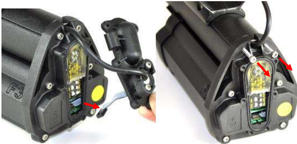
Figure 50: Disconnecting wiring loom.
